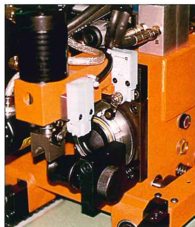
2 • Carriage with lifting device which allows the processing of pipes longer than the machine's maximum capacity when working without the mandrel rod.
